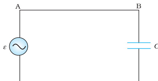
FIGURE 7.8 An ac source connected to a capacitor.
