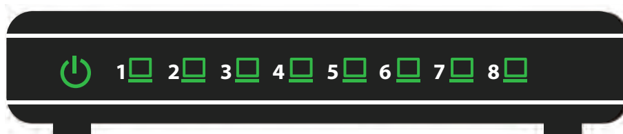
Figure 5.8: A network hub with 8 ports
