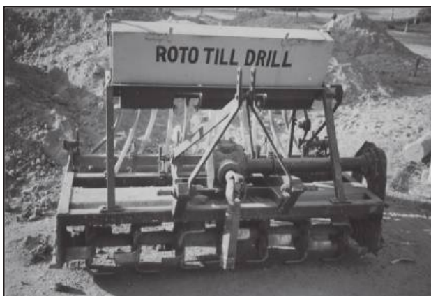
Fig. 5.12 : Roto Till Drill—A modern agricultural equipment
