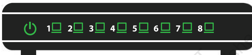
Figure 10.11: A network hub with 8 ports
