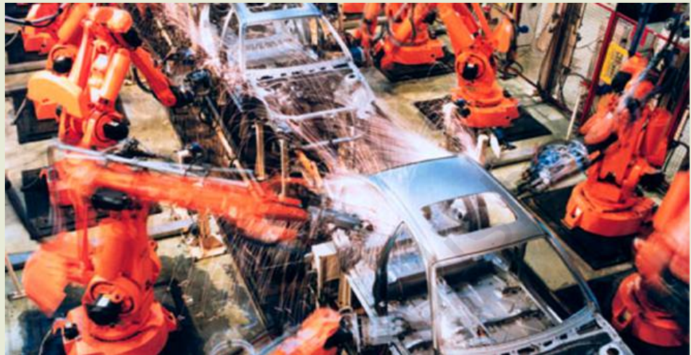
Figure 14.6 : Robot welding the car body
