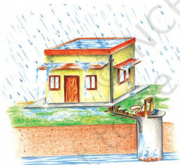
(b) Recharge through Abandoned Dugwell
