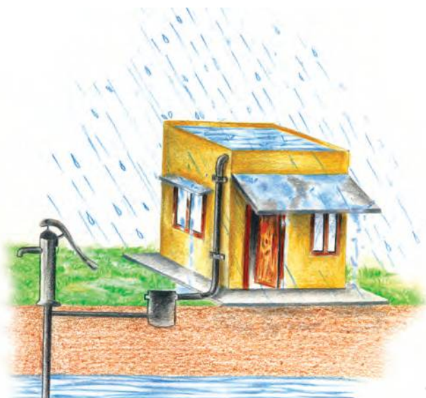
(a) Recharge through Hand Pump
