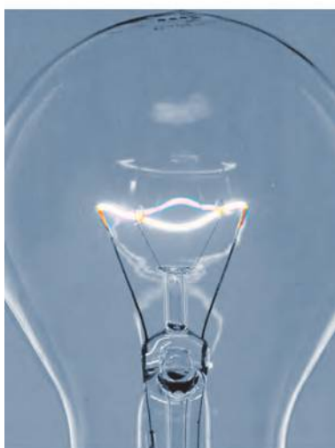
Fig. 14.12 Glowing filament of an electric bulb (incandescent)
