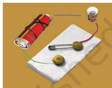
Fig 12.9 An electric circuit with a switch
