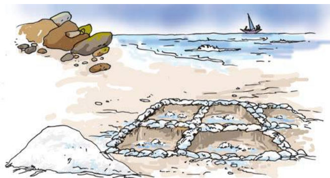
Fig. 5.12 Obtaining salt from sea water
